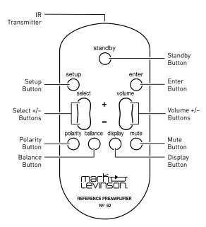
*IR transmitter:* This transmitter sends infrared signals to the IR receiver on the Controller's front-panel display
