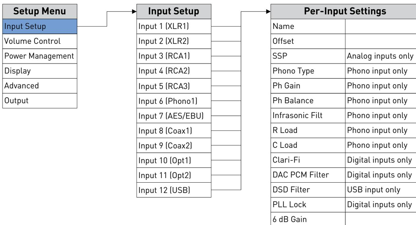
The Input Setup menu allows you to customize the following parameters for the selected input:
