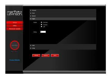
**Trigger:** This setting configures the 12V trigger. NOTE: Using a trigger input overrides the *Standby* button.
