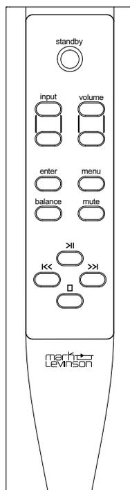
**Standby:** Press this button to put the N°5206 into and out of the *Standby* mode. Press this button twice to wake up unit from green *Standby* mode.
