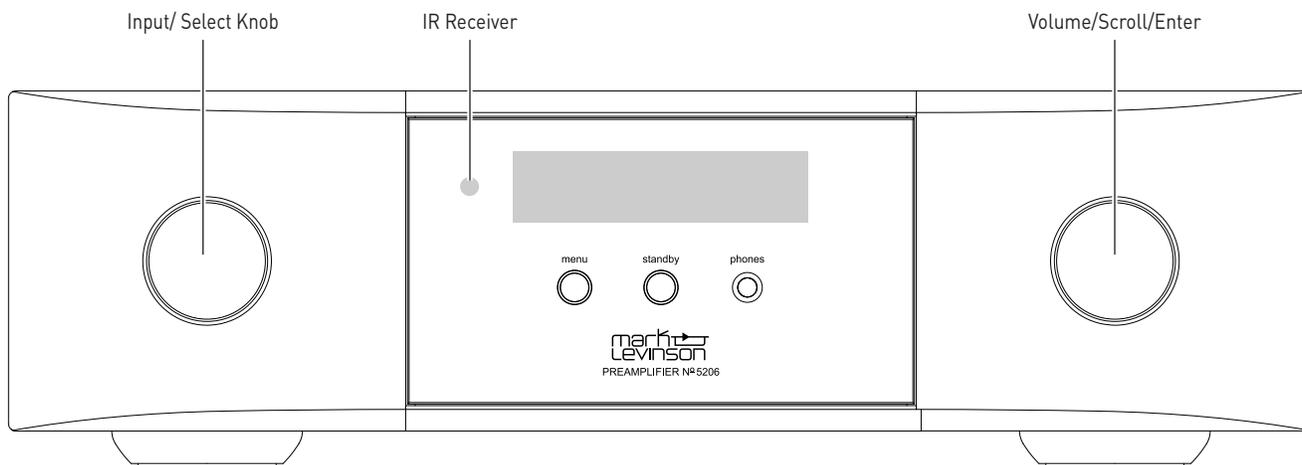
The Mark Levinson team designed the N°5206 for elegant simplicity and ergonomics; therefore, the knobs perform a variety of functions depending on the operating mode. There are two modes of operation, *Listening* mode and *Setup* mode, and three modes of *Standby*, Green, Power Save, and Normal.
