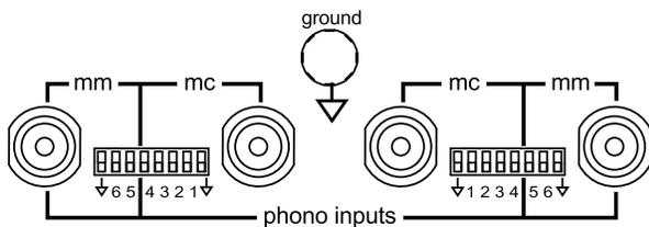
The phono inputs are balanced. Setting the ground switch ↓ to the *up* position references the input to ground which is sometimes useful if there is excessive noise or hum present. Be sure to use the ground switch designated for the connected input.
