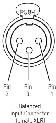
Balanced connector pin assignments:
